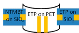
Figure 8. Schematic illustration of a prototype that is able to sense temperature, RH and load using different substrates (PET substrate in the center and silicon oxide substrates in sides) and 2 different MCNPs. The gold lines represent the metal electrodes.
